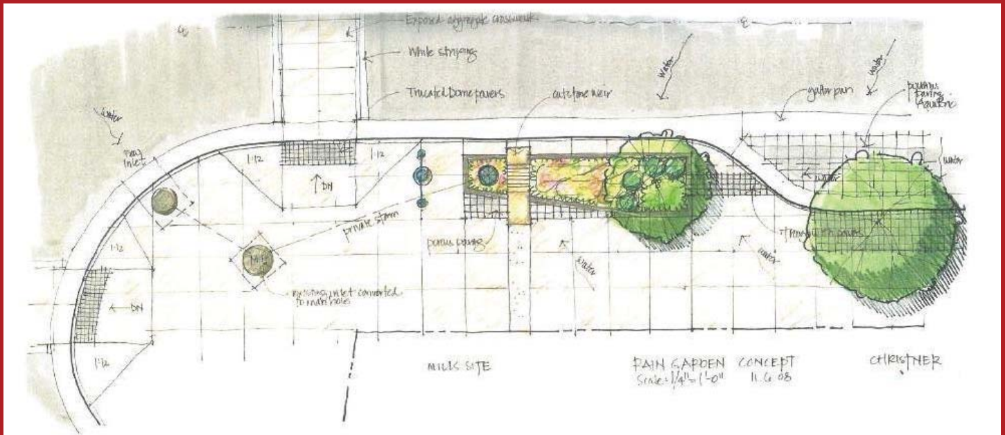
Rain Garden Concept – storm water from porous paving enters the planted rain garden from the curb side and is cleaned, reduced in volume and retained.
